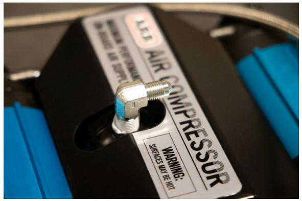
Then, connect the air line to the flared end of the 90 degree fitting like the photo below. Ensure all of the fittings are tight to prevent air leaks. The flared fittings do not require thread tape. Adding thread tape to the flared fittings will prevent a proper seal.
